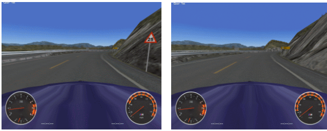
Figure 3: The dynamic speedometer shown on the right of the screen changes from 40 mph to 25 mph as soon as the driver goes past a speed limit sign in the driving simulator.
