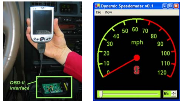
Figure 4 - In-car prototype showing the OBD-II interface and the visualization used for the dynamic speedometer.
