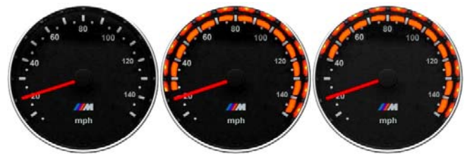
Figure 2: a) Standard speedometer, b) Dynamic speedometer showing 25 mph speed limit, c) Dynamic speedometer showing 40 mph speed limit
