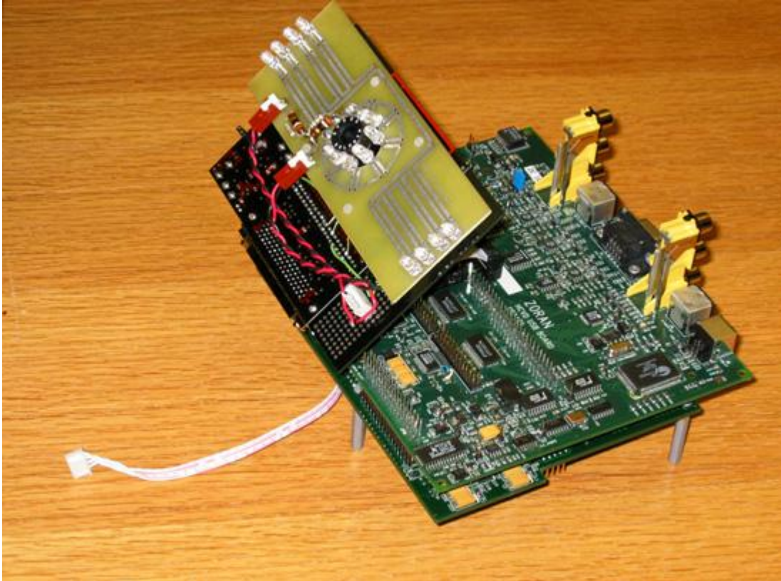
Figure 59. Amir et al.'s prototype of a hardware eye-detection sensor. Image processing is done on an on-board FPGA, making this a lightweight peripheral that can be connected via USB.
