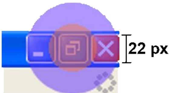
Figure 11. Confidence interval of eye tracker accuracy. Inner circle is 0.5^\circ . Outer circle is 1.0^\circ .
