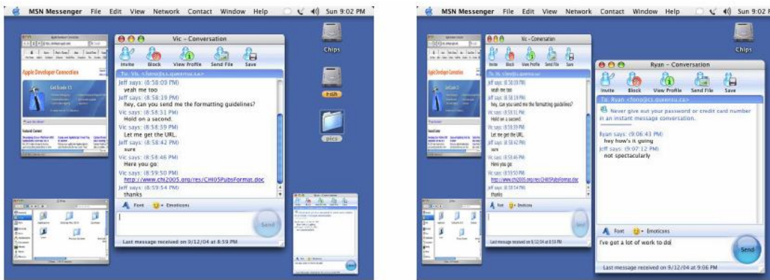
Figure 34. Fono et al.’s EyeWindows technique for switching between non-overlapping windows using eye gaze. When the user looks at a particular window, it is restored to its full dimension while all other windows are distorted using an elastic windowing algorithm.
