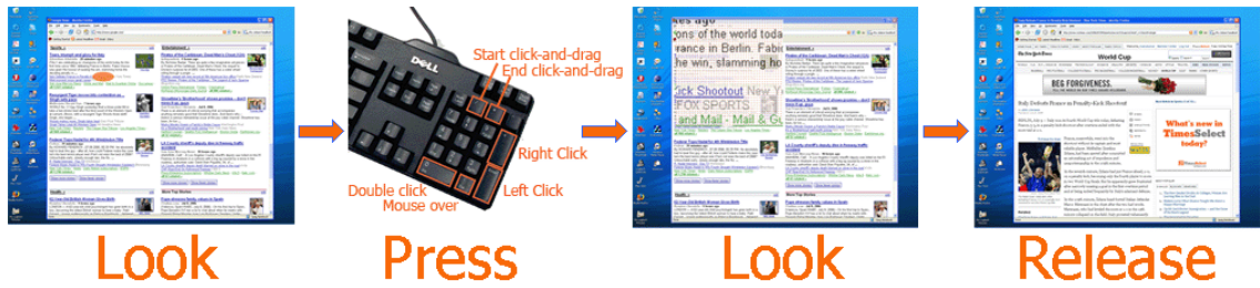
Figure 14. Using EyePoint for a progressive refinement of target using look-press-look-release action. The user first looks at the desired target. Pressing and holding down a hotkey brings up a magnified view of the region the user was looking in. The user then looks again at the target in the magnified view and releases the hotkey to perform the mouse action.
