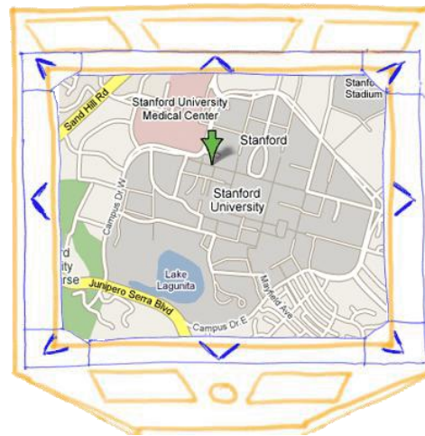
D. 8-way panning regions activated by looking slightly off-screen for a micro-dwell duration (150-200ms)
