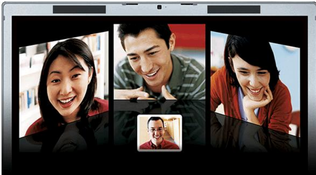
Figure 60. Concept eye tracker — here the Apple MacBook Pro has been shown with two black bars in the top bezel, which can conceal the infrared illuminants necessary for eye tracking.
