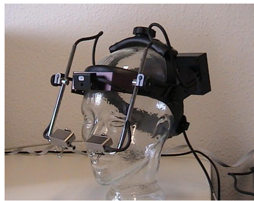
Figure 6. A head mounted eye tracker which fixes the position of the camera relative to the motion of the head.
