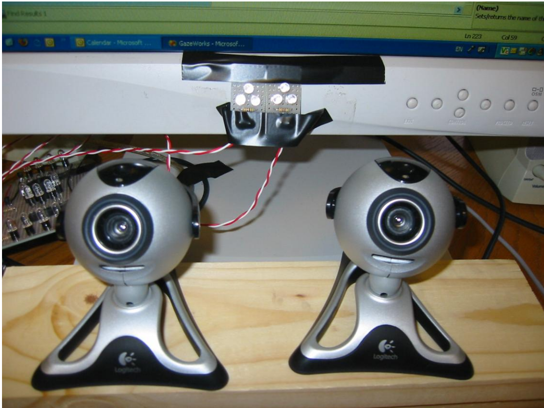
Figure 57. The low-cost prototype in development uses commercial-over-the-shelf cameras modified to work in the infrared spectrum. The glint source pictured above uses IR LEDs (invisible to the human eye).
