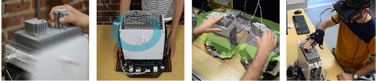
Figure 1. shapeShift is a mobile tabletop shape display that enables 2D spatial user input and output. Left to right: (a) In passive mode the user can freely move the display; (b) The display serves as a spatially-aware physical lens into underlying information; (c) Two displays can be used to simultaneously explore different regions; (d) In active mode shapeShift can move on-demand - here it tracks the user's hand to simulate the presence of virtual content
