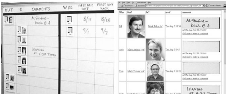
Figure 2. Collaborage (Moran et al., 1999), a spatial TUI where physical walls such as an in/out board (left) can be captured for online display (right). Reproduced with permission.
