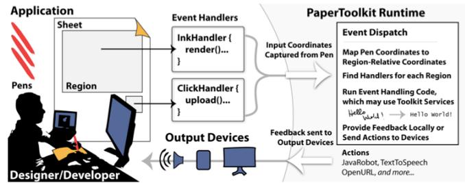
**Figure 2.** In PaperToolkit, input arrives from pens (left) and is sent to handlers (middle). Output is displayed on the local machine or routed to devices (bottom). Event dispatch and UI construction are modeled after GUI architectures, to help programmers create paper + digital applications rapidly.
