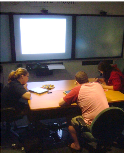
Figure 2. The collaborative sketching system affords simultaneous input to and viewing of a shared sketching space (top) through networked Tablet PCs and a digital whiteboard (bottom).
