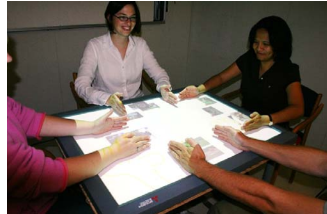
figure 1. Four users execute a cooperative gesture to organize digital documents on an interactive table.
