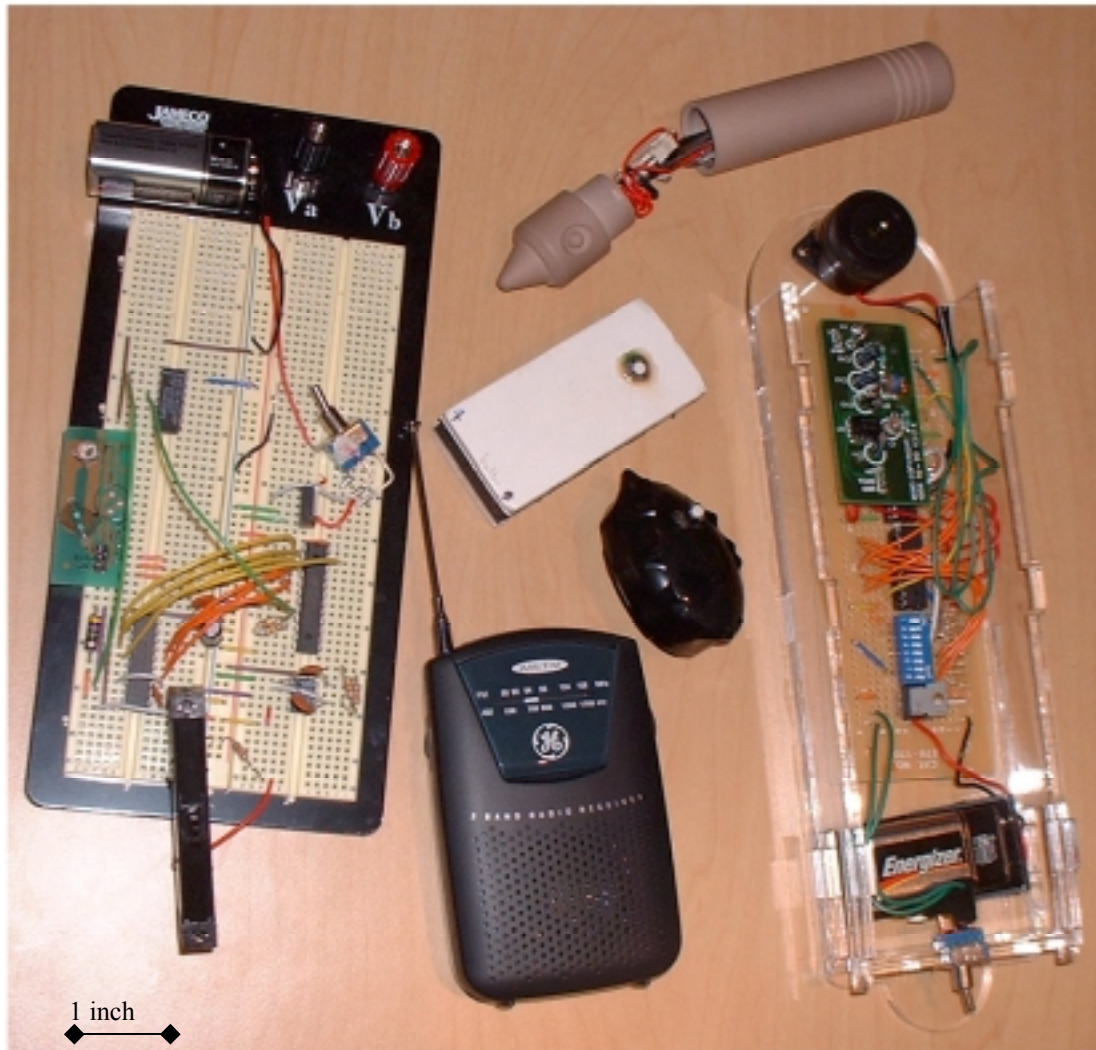
Figure 3. The various types of iStuff created so far—buttons, potentiometers, speakers, and buzzers.
