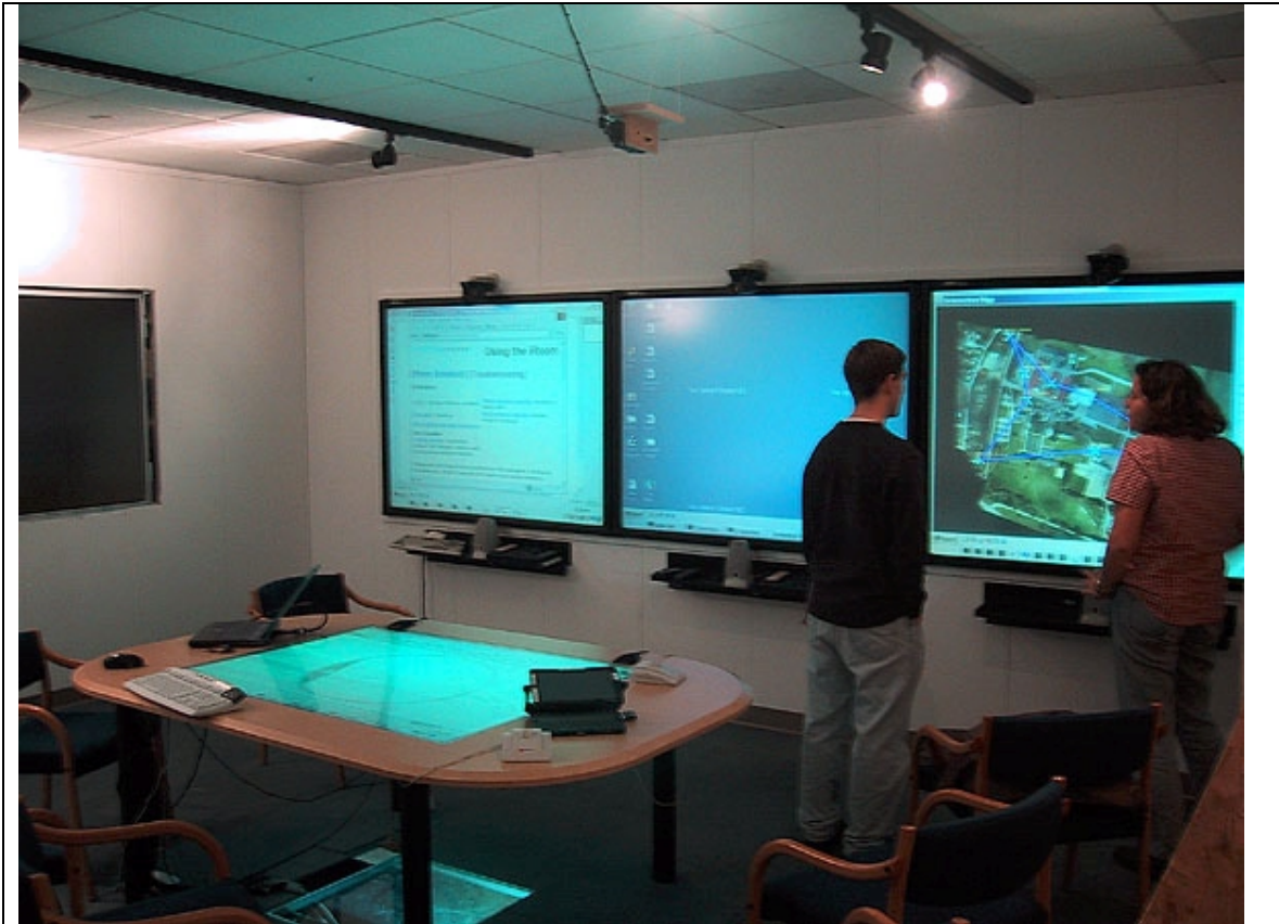
Figure 1. The Stanford iRoom contains a wireless GyroMouse and keyboard (visible on the table), three touch-sensitive SmartBOARDS and one non-touch-sensitive tabletop display, and a custom-built OpenGL hi-res graphic mural. The room is networked using IEEE 802.11b wireless Ethernet. Except for the hi-res mural and the tabletop, all hardware is off-the-shelf, all operating systems are unmodified Windows (various flavors) or Linux, and all software we have written is user-level.
