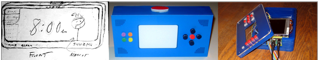
Figure 3 A paper sketch, physical mock-up, and final prototype (implemented with d.tools), showing how the interface of SnuzieQ, an alarm clock, evolved through prototyping.
