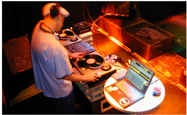
Figure 8 Final Scratch: encoded vinyl for digital music.
