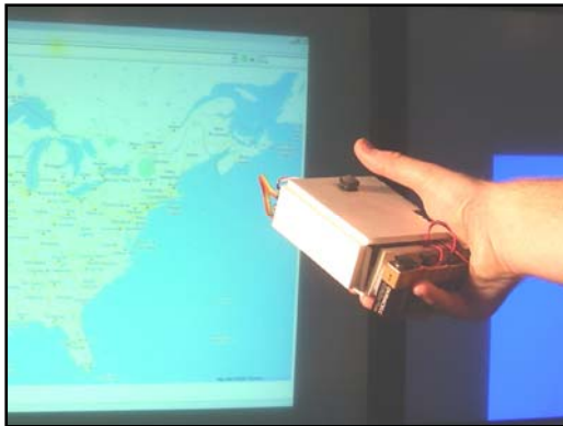
Figure 2: The tilt-sensing Google Maps navigator.
