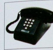
1963: Bell Labs introduce the touch-tone telephone to replace rotary dial telephones. This paves the way for telephone services such as short text messaging.
