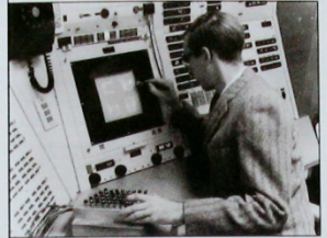
1963: Ivan Edward Sutherland invents the Sketchpad , which makes it possible to create graphic images directly on to a display screen via the use of a hand-held object such as a light pen.
