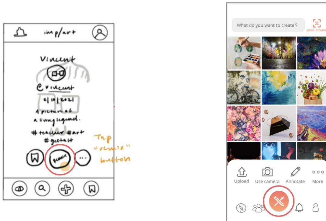
Fig. 15. Low-fi (left) vs Medium-fi (right) designs for posting to Peek, with the post buttons for each prototype circled in red.
