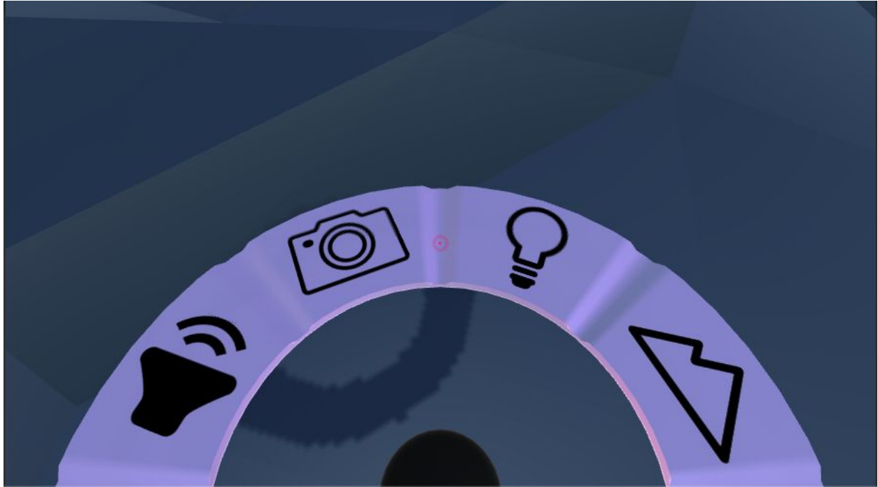
(Fig. 4.3) 360-degree radial menu as seen in virtual reality. Visible buttons: add sound, add media, add light, change terrain.
