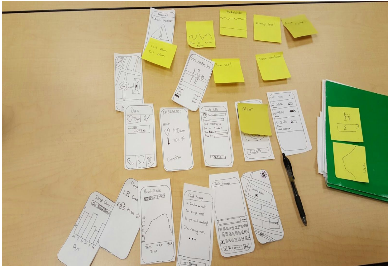
This is an overview of all 14 screens. We used sticky notes to model transitions between screens.
