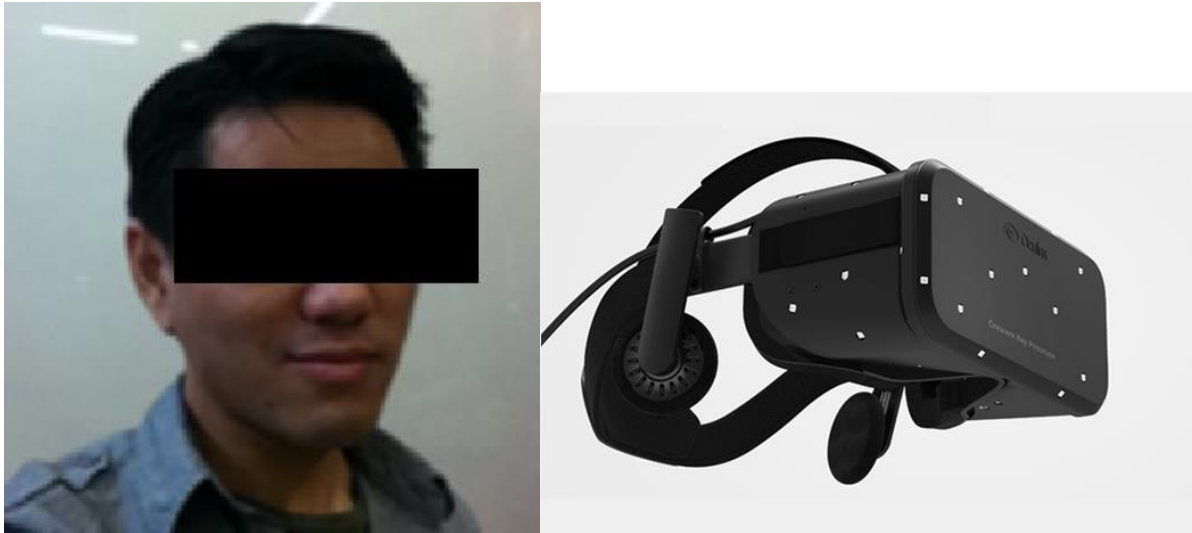
Figure 8. Crescent Bay , the latest prototype of the Oculus Rift. This head-mounted display features LEDs on both the front and back to allow for positional tracking even if the user is turned and not directly facing the camera that Oculus provides.
