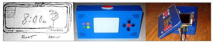
**Figure 3** A paper sketch, physical mock-up, and final prototype, showing how the interface of SnuzieQ, an alarm clock, evolved through prototyping.
