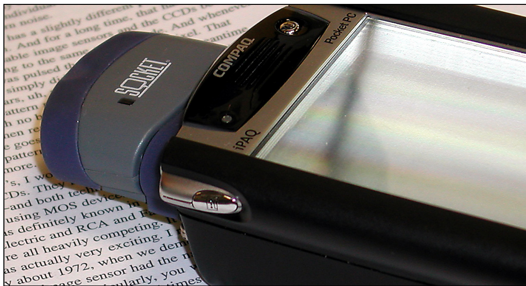
FIGURE 6.6 The trigger button initiates barcode scanning.
