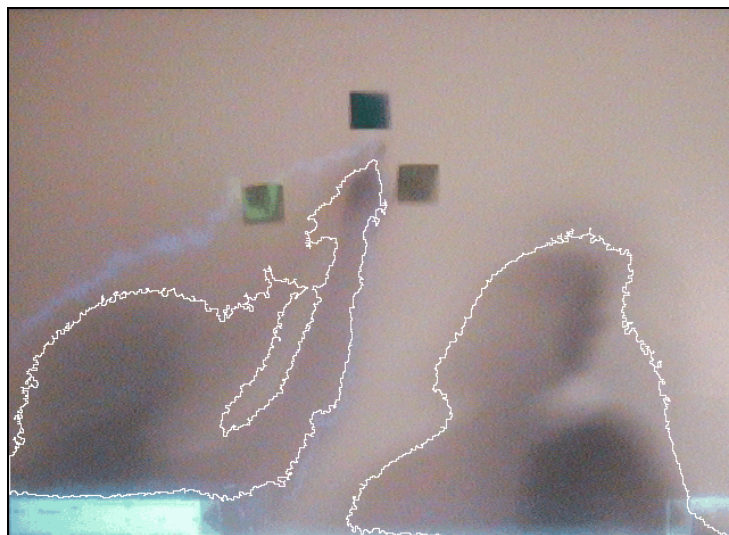
FIGURE 5.8 The view from the rear camera of two users, one of whom is pointing to a note on the board. The calculated borders of the shadows are drawn in white, on top of the raw pixel input.
