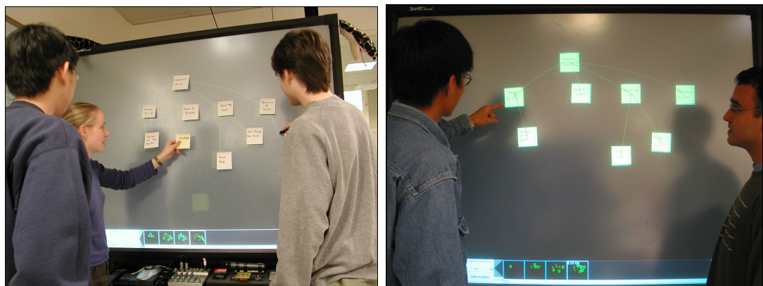
FIGURE 5.1 Our remote system running on two SMART Boards. Notes that are physical in one place (see left) are electronic in the other (at right). The Outpost history bar at the bottom shows previous states of the board.
