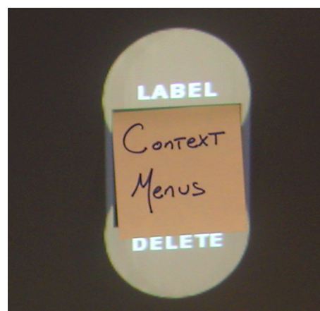
FIGURE 3.12 Tapping on a note invokes an electronic context menu for physical content.
