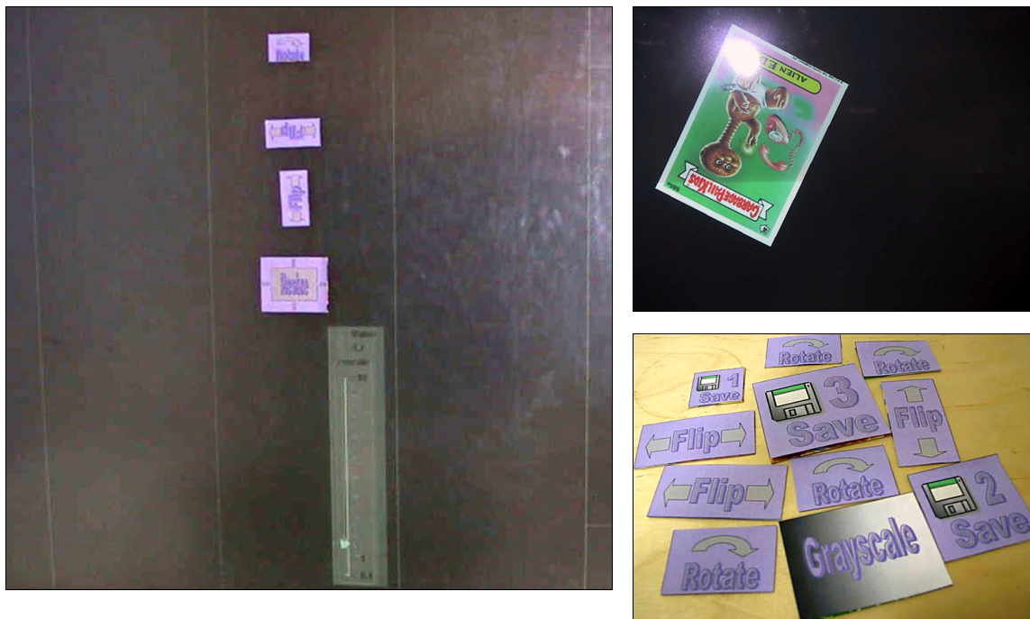
FIGURE 9.1 The Physical Macros class project: a wall-scale, topological TUI. At left , a set of physical operation cards placed on the SMART Board; the resize operator is parameterized with an electronic slider. At top right , the image resulting from the operations. At bottom right , the set of physical operation cards available to the user.
