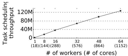
Figure 5: Canary scheduling throughput grows almost linearly with the number of workers, reaching 127M tasks/sec with 64 workers (1,152 cores). The high throughput allows jobs to be split into as many tasks as needed without concern for the scheduler overhead.
