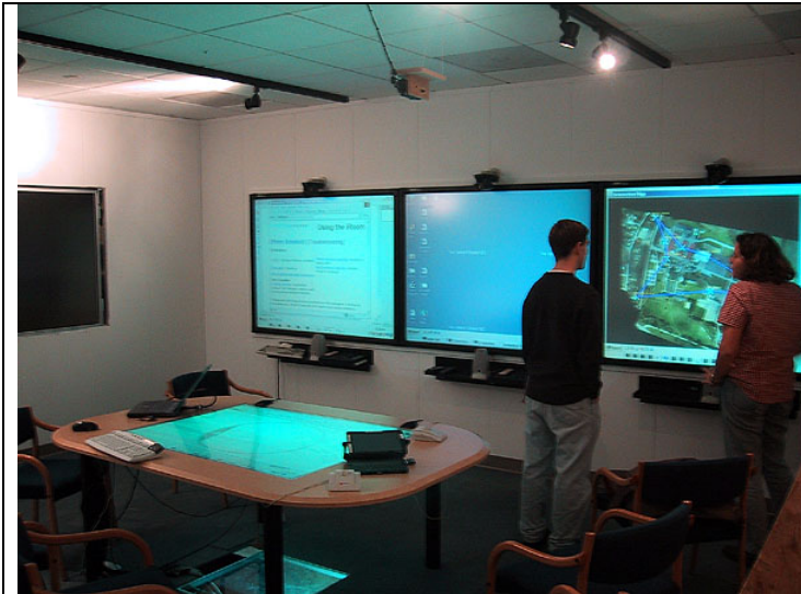
Figure 2 - A View of the Interactive Room v2 (iRoom). The hi-res Mural, visible at far left, is mounted in a wall that was used as a passive projection surface in our original iRoom. The orientation of the space was also rotated 90 degrees relative to the original iRoom, requiring compact light-folding optics for the three SMART Board rear-projected displays.
