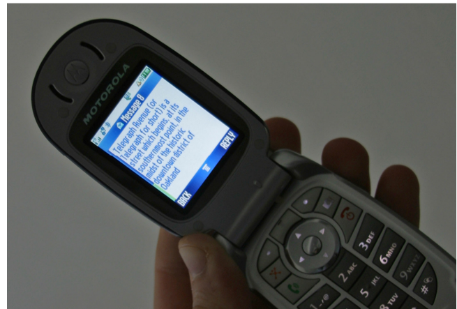
Figure 1. The low-fidelity, ‘Wizard of Oz’ prototype on a Web-enabled cell phone, Motorola V551
